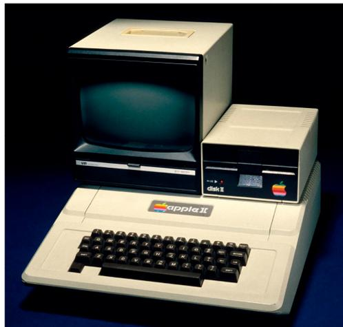
Figure 1.2: An Apple II computer with an integrated keyboard (presented in 1977). Taken from [240].
