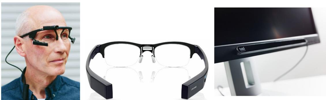
(a) A wearable eye tracker using infrared cameras to observe the eyes. Taken from [236].
