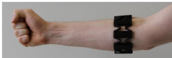
Figure 4.4: A user wearing the Myo and currently holding a control by making a fist and adjusting it by rotating the arm.
