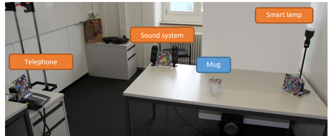
Figure 2: The setup of connected smart devices used for the study consisting of a lamp, a sound system, and a phone. The mug used in scenario 3 is also shown. In our prototype, all have an individual marker attached for visual recognition.
