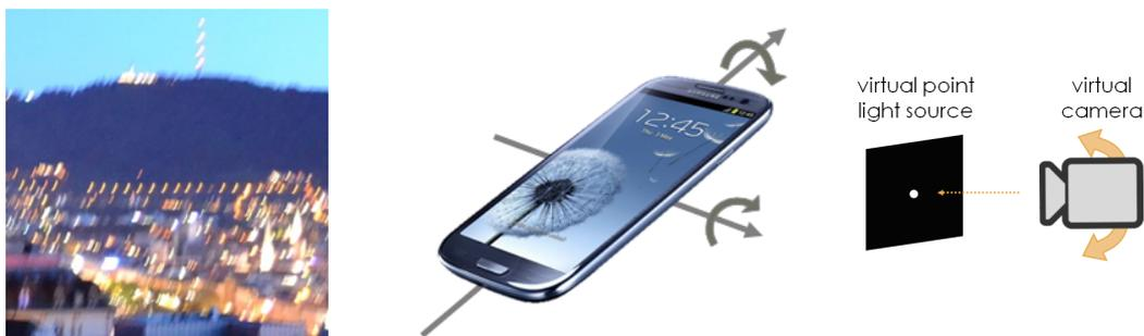
Figure 3.27: Left: The blur is “encoded” in the image of point light sources. Middle: We can reconstruct the camera motion from inertial sensor measurements. Right: We can get the blur kernel by replaying the motion with a virtual camera looking at a virtual point light source.
