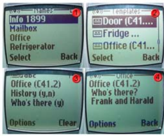
Figure 1: Phone book entries (1) and a list of SMS templates for smart objects (2), an edited SMS template with activated command (3), and the response SMS message (4)
