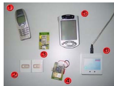
Figure 2: Some of the devices used in the experiments – a Bluetooth-enabled mobile phone (1), RFID tags (2), a Bluetooth access point (3), a Smart-Its (4), a Bluetooth-enabled iPAQ (5), and an RFID scanner (6)
