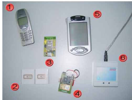
Fig. 1. Some of the devices used in the experiments — a Bluetooth-enabled mobile phone (1), RFID tags (2), a Bluetooth access point (3), a Smart-Its (4), a Bluetooth-enabled iPAQ (5), and an RFID scanner (6)
