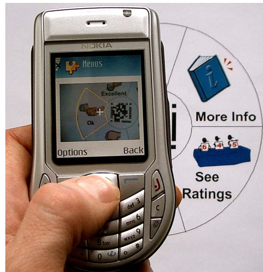
Figure 1. A user interacting with a printed visual code pie menu. On the phone screen, the focused pie slice has a yellow frame.
