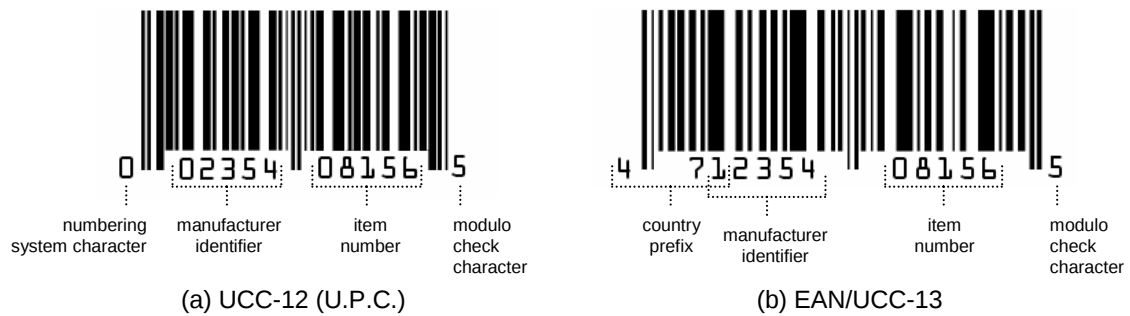
Figure 8.2: Global trade item numbering structures: (a) UCC-12 (U.P.C.) and (b) EAN/UCC-13.
