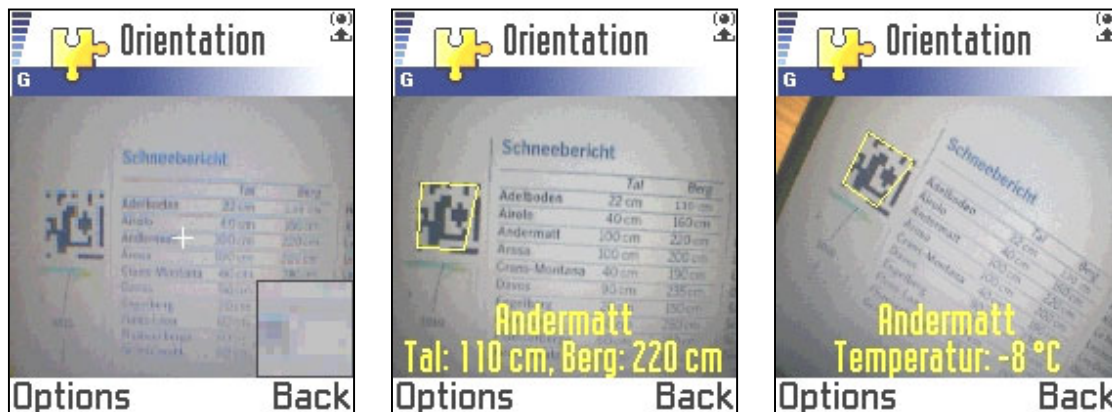
Figure 3.12: Selection from a table: the code coordinates determine the table row, the camera rotation specifies the concrete information aspect to display.
