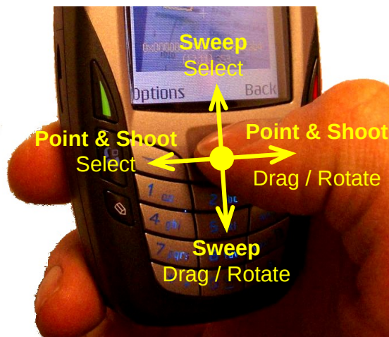
Figure 6.5: Phone input interaction: point & shoot is mapped to horizontal joystick push-and-release, sweep is mapped to vertical push-and-hold.
