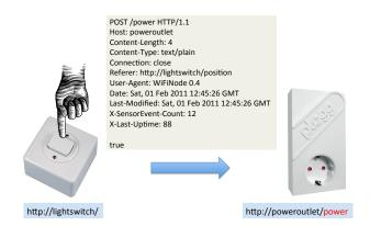
Figure 3: Connecting things using HTTP callbacks
