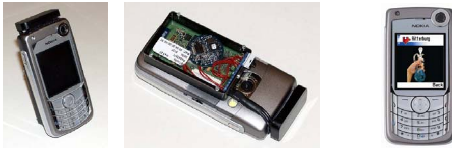
Fig. 10. Mobile phone with RFID-reader and external antenna (a) front and (b) back view; and (c) mobile phone that embodies the role of a magic potion
