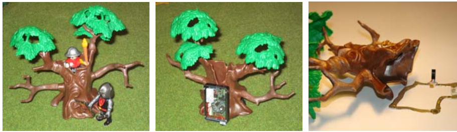
Fig. 9. (a) Enchanted tree, (b) with mobile RFID reader and (c) with custom-built antenna
