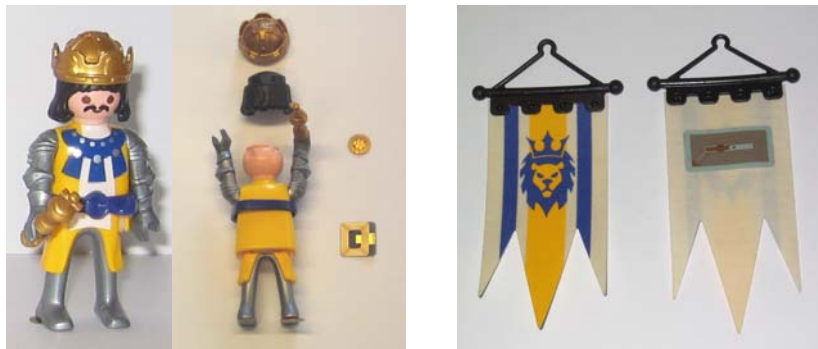
Fig. 8. (a) Figure of king with RFID tags, (b) Flag of castle with RFID tag
