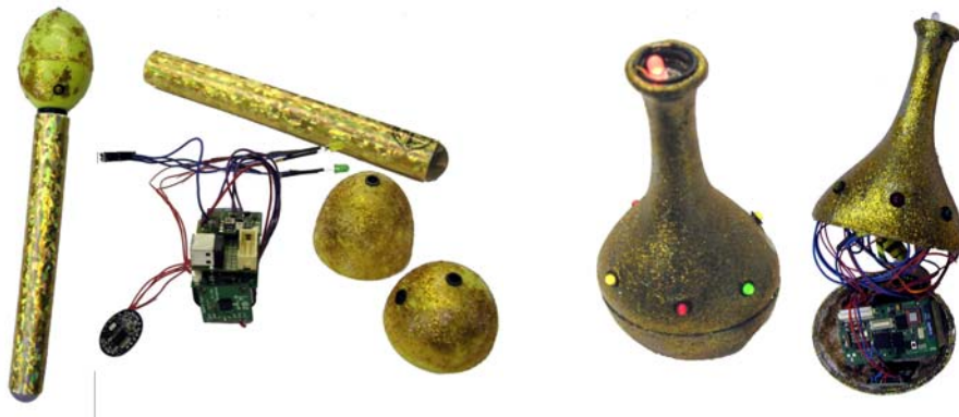
Fig. 11. BTnode with RFID reader and sensor board embedded into a toy wand and bottle
