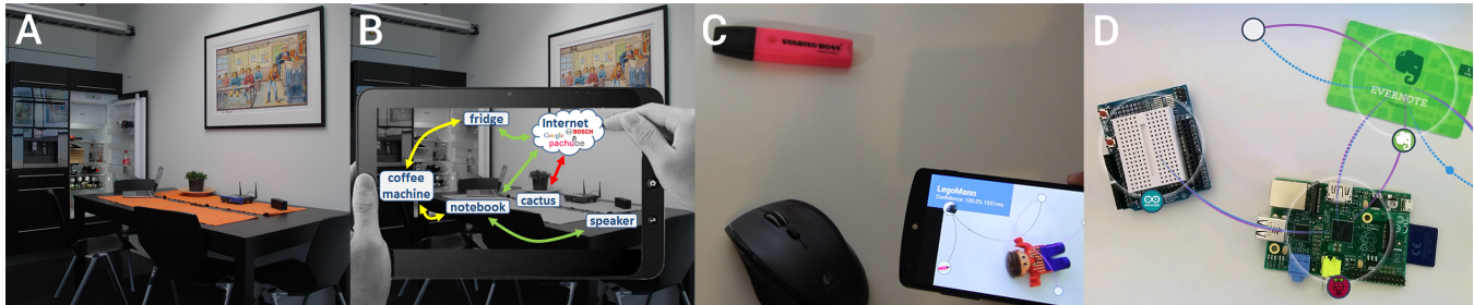
Figure 1: A magic lens for visualizing communication links in smart environments. A) and B) Idea: Users can reveal communication links by observing devices through a tablet computer. C) and D) Screenshots of our tool showing messages being passed between connected objects.
