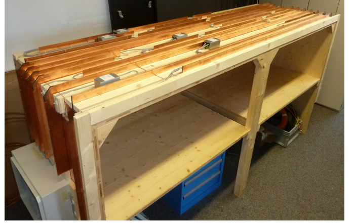
Fig. 2. Test bench design: Isolated copper corridors are used to create long wire lengths
