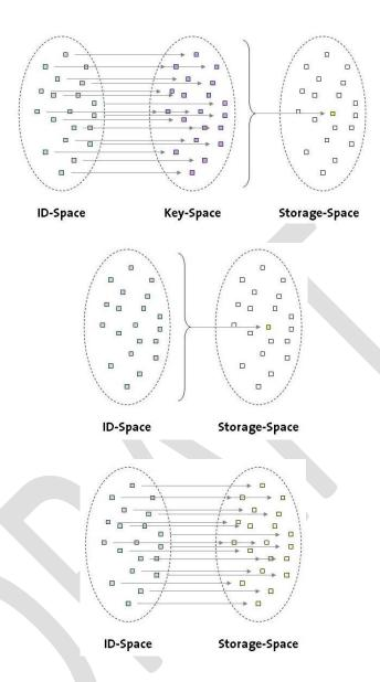
• Figure 6: ID-storage mapping options. In the FragDB prototype, each ID points to a data share, fragmented within the database and only accessible through the individual IDs (bottom). One could, however, also envision a set of tags pointing to a single memory location, e.g., identified by a single URL (middle), or the fragmented data itself allowing the reassembly of such a URL (top).
