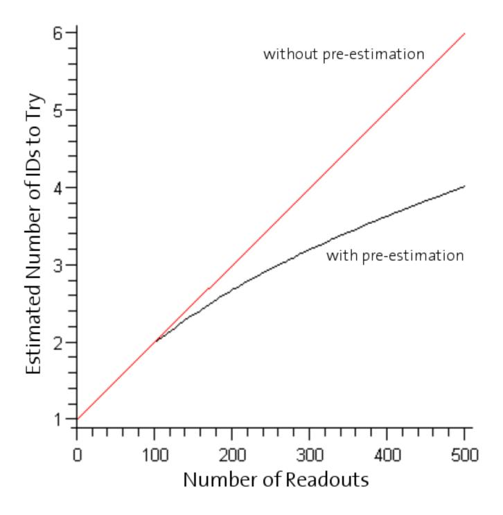
• Figure 11: Payoff from estimating the correct number of ID changes. Knowing how often a tag changed its ID can lower the number of IDs that need to be tried before the correct fragment can be found. The above graph uses p=1% and no ID-fading.
