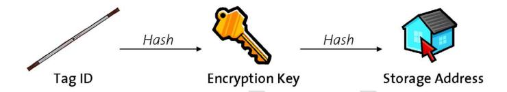
Figure 8: Derivation of Storage Address and Encryption Key. The tag ID is not used directly to store the data, but repeatedly hashed to derive the encryption key of the fragment data, which in turn leads to the storage address of the encrypted payload.
