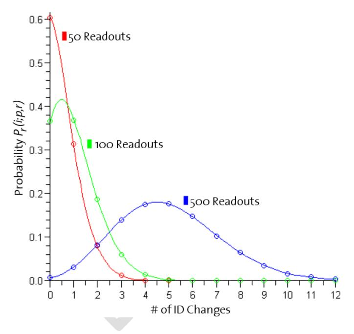
• Figure 10: Binomial distribution of ID-changes for an ID-change probability of p=0.01 and a number of different readouts (50, 100, 500). The more readouts are made, the flatter the curve becomes, thus making it harder to correctly guess the number of ID changes.
