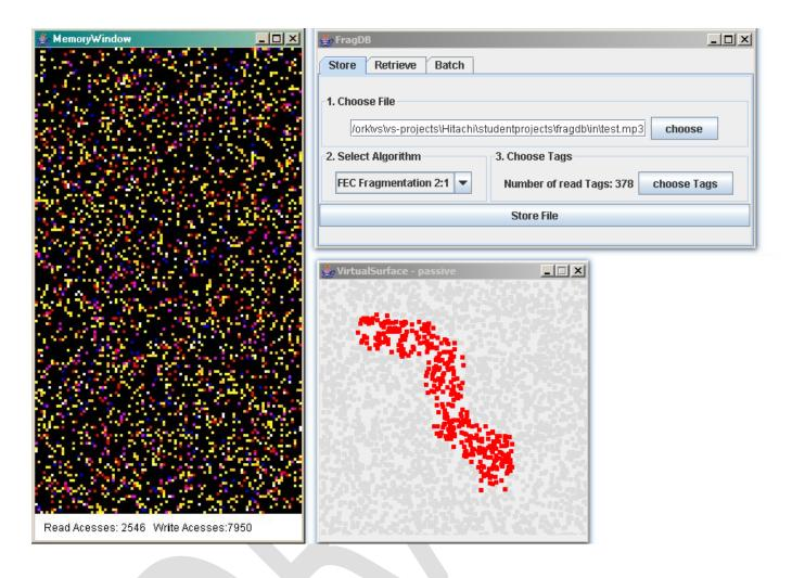
• Figure 2: Prototype interface. The FragDB Prototype is used for both simulating large tag populations (using a simulated surface with embedded tags as shown in the window "virtual surface"), as well as directly controlling a physical reader device. A "memory window" shows read and write access to a virtual storage system.
