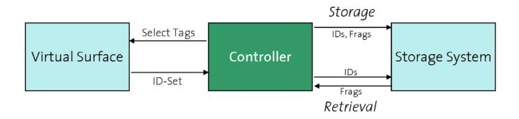
• Figure 5: FragDB Controller. The controller receives a set of tag-IDs from the simulated surface ("virtual surface"). It uses this to either store a fragmented file in the storage system ("storage") or to retrieve a set of corresponding fragments from it ("retrieval").
