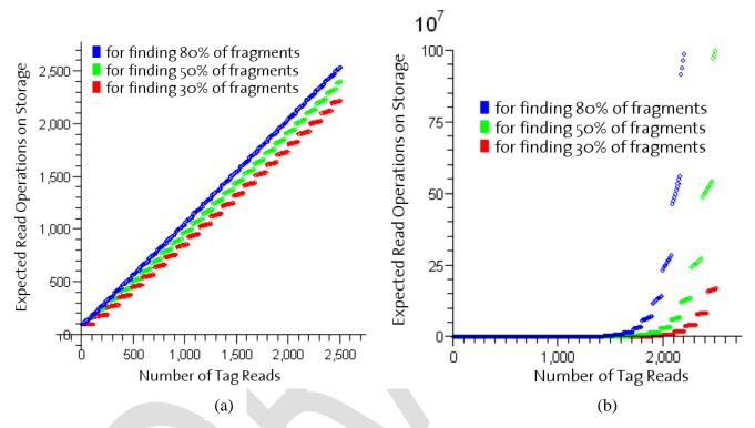
• Figure 12: Maximum reads requests for 100 tags. Subfigure (a) shows the number of expected read operations without ID-fading. Access to the storage system grows linearly over time – sudden jumps are due to ID-updates on the tags. Subfigure (b) shows the effect of enabling ID-fading. Retrieval quickly involves millions of storage accesses after a few thousand read operations. Note the different scale of the y-axis.
