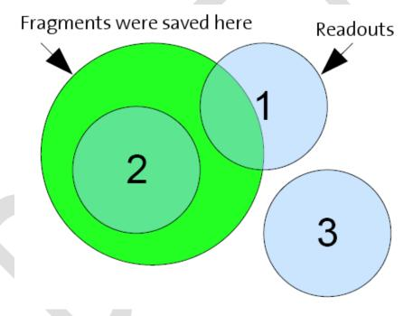
• Figure 13: Choosing the right tag set. When reading a location at a later time, the reader might not correctly catch the exact set of tags that were used during saving. In the above example, case 1 only partially overlaps, case 2 catches only correct tags, but not enough, and case 3 is totally off.
