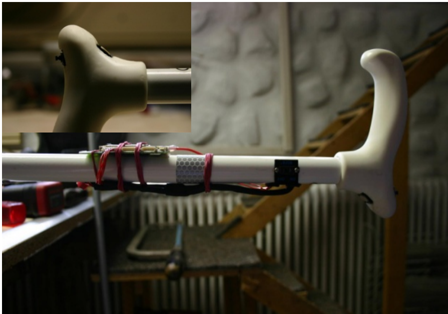
Figure 7.14: The “smart cane,” with the two command buttons (five-way navigation and dedicated select button) on the handle, an on-off button below, and the BTnode for Bluetooth command transmission further down. The batteries for the operation of the BTnode are hidden inside the cane’s shaft. The picture’s upper left corner shows a close-up of the two buttons for logical navigation on the handle.
