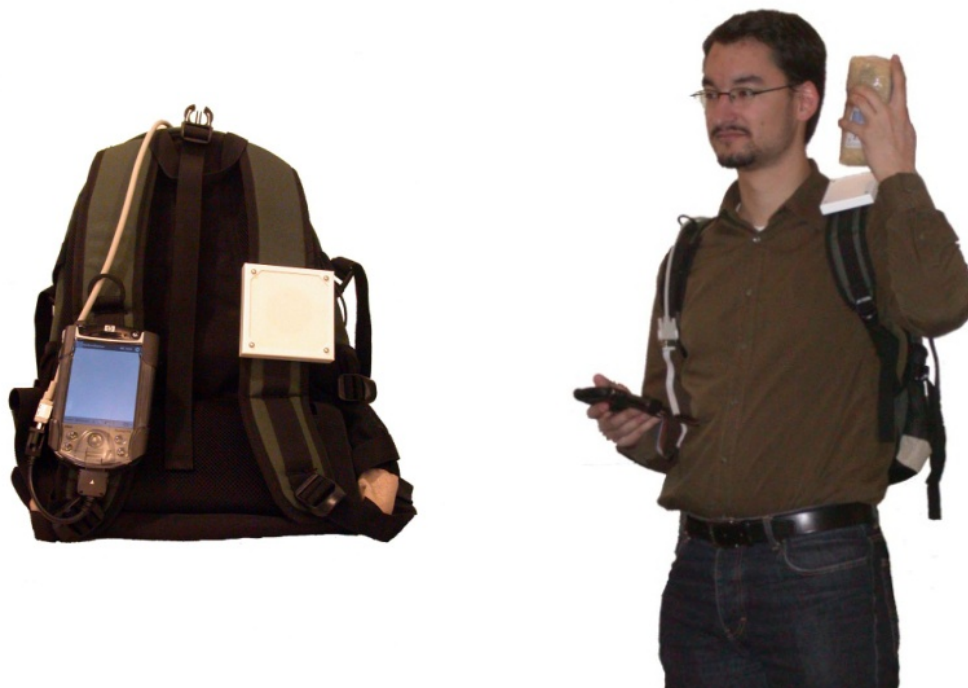
Figure 7.13: The usability solution for a system comprising both motes and RFID tags. On the left, the backpack containing the mote base station and the RFID reader. On its outside, the RFID antenna (left shoulder) and the mobile device (right shoulder). On the right, a typical usage of the system to scan a supermarket product for additional information.
