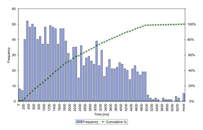
Figure 3: Average time to establish a connection with a device that is in inquiry-scan mode
