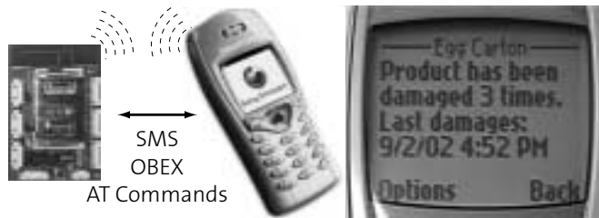
Figure 8. Product monitoring using BTnodes as smart tags and SMS via mobile phones
