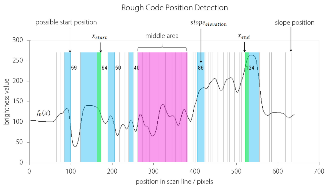
Figure 3.17 Detection of the approximate code start and end position.
