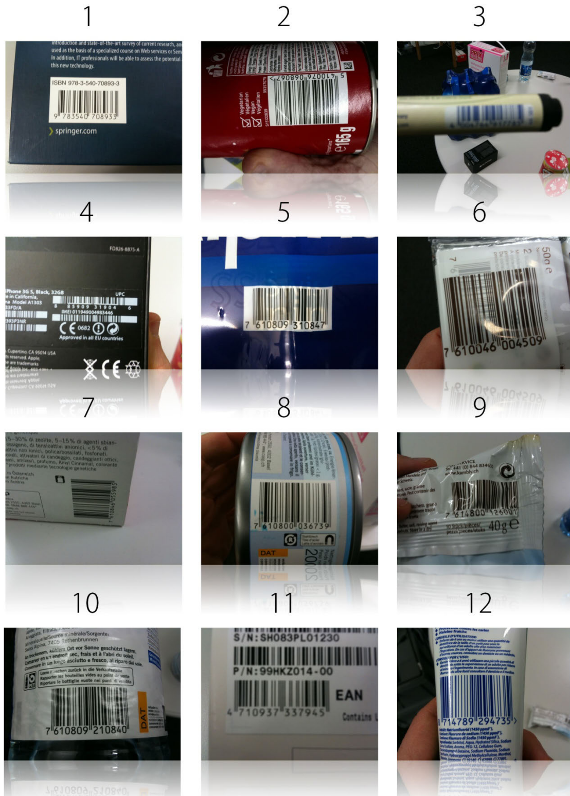
Figure 5.2 Test products: Easy-to-recognize code (1), normal bar code that was often scanned upside-down (2), colored and thin bar code resulting sometimes in blurry images (3), thin and multiple codes (4), code on non-straight and slightly transparent surface (5), slightly crumpled and transparent code frequently exhibiting glare (6), code on heavy product that was often scanned from an angular perspective (7), small code (8), crumpled code with often occurring glare (9), code on round surface (10), multiple codes (11), code on non-straight surface with frequently occurring glares (12).
