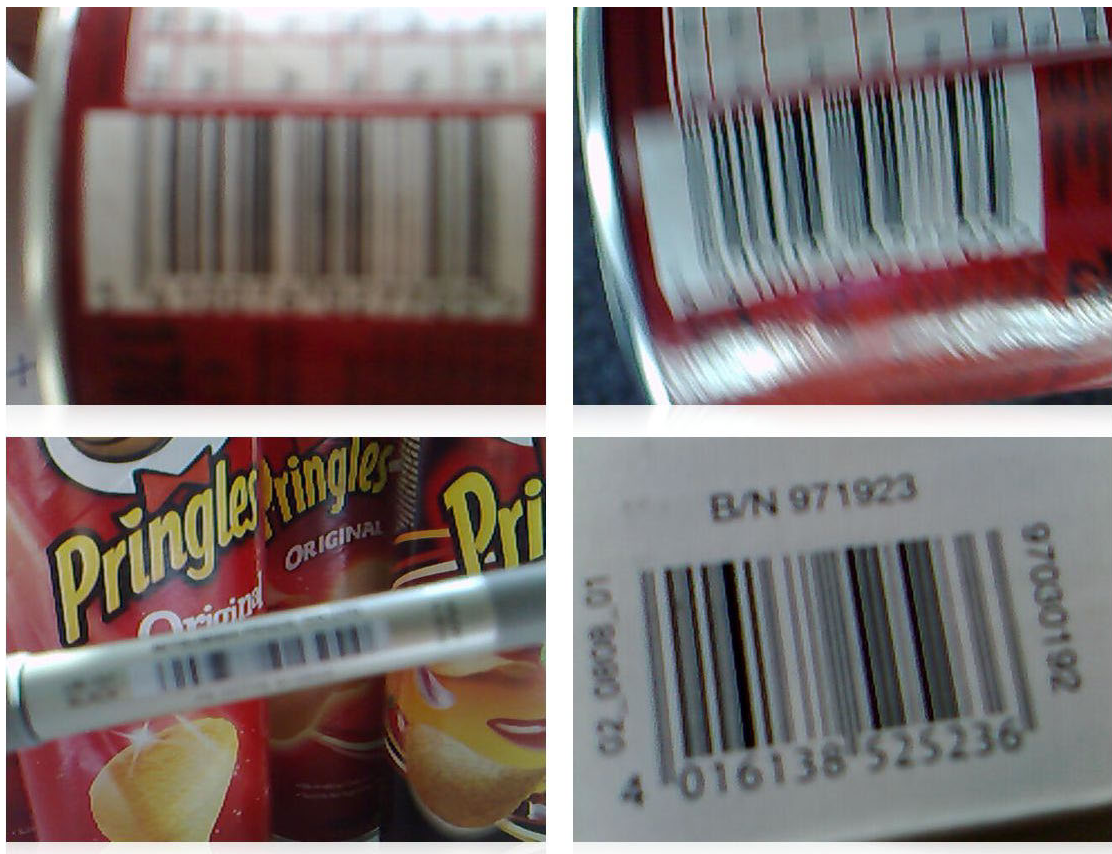
Figure 2.1 Examples of blurry images: Out-of-focus blur on device without AF camera (upper-left image), blurry image due to hand movements (upper-right image), blurry image due to wrong focus point (lower-left image), and slightly blurry image because the AF camera can't focus on too close objects (lower-right image).
