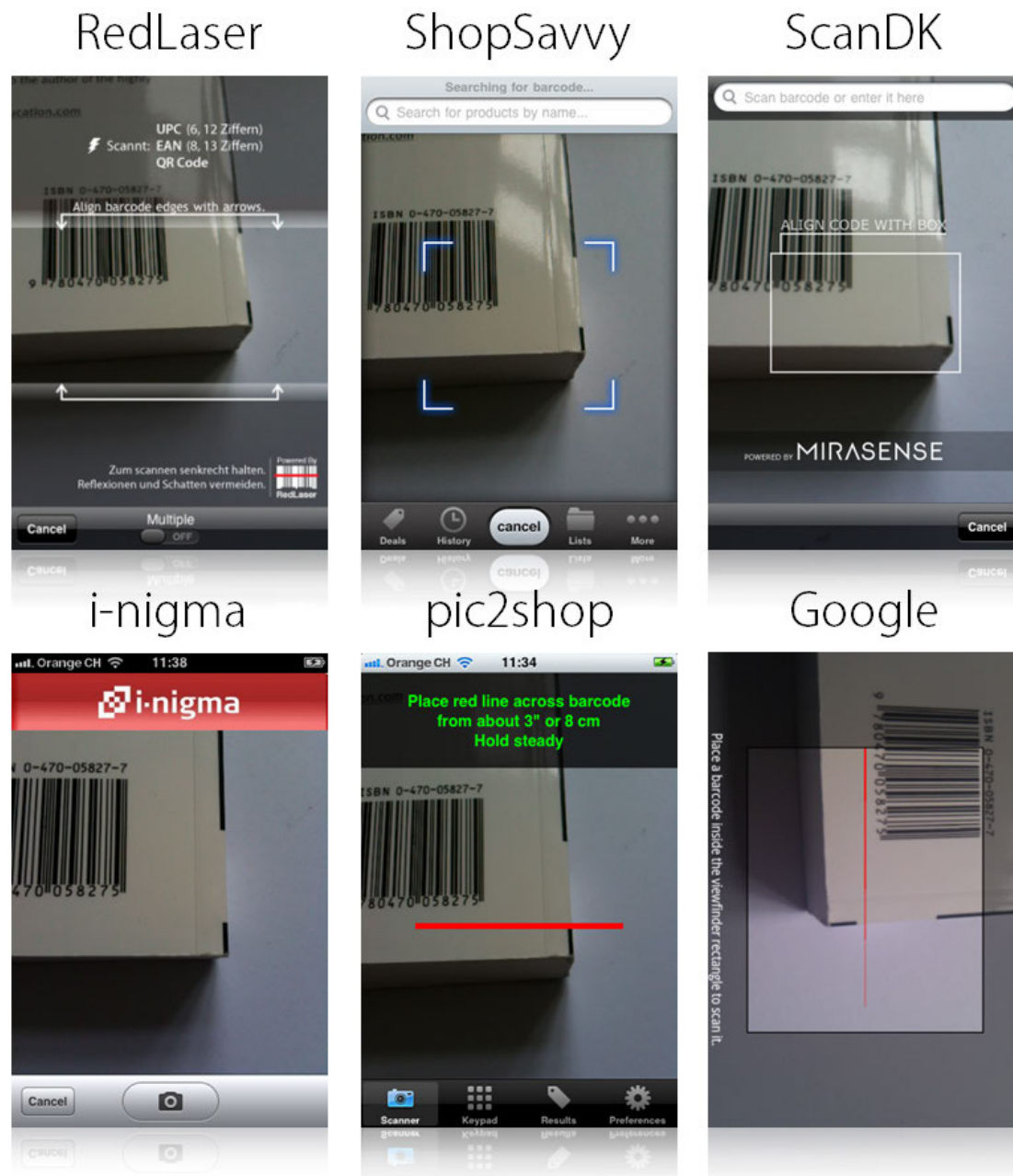
Figure 5.12 User interfaces of scanners tested in the user-study. Interface types include rectangle-shaped (RedLaser, ShopSavvy and ScanDK), scan line-shaped (pic2shop, Google) as well as no (i-nigma) viewfinder elements.
