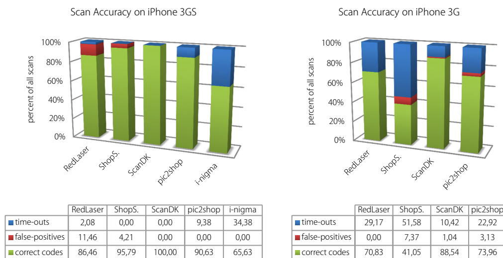
Figure 5.6 Results scan accuracy on iPhone 3GS (left image) and iPhone 3G (right image) for easy-to-recognize test products.
