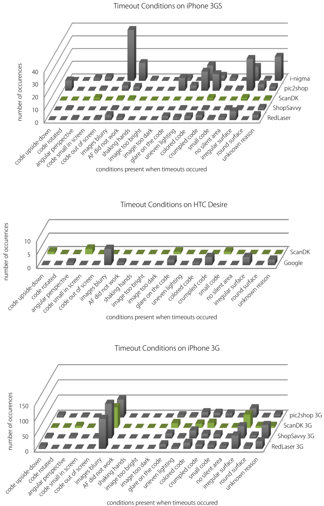
Figure 5.13 Prevailing conditions in case of time-outs for the different scanner applications and mobile phones. In case of the iPhone 3GS it is visible that although the mobile phone has a built-in autofocus camera, i-nigma could often not recognize a code because the image was blurry.
