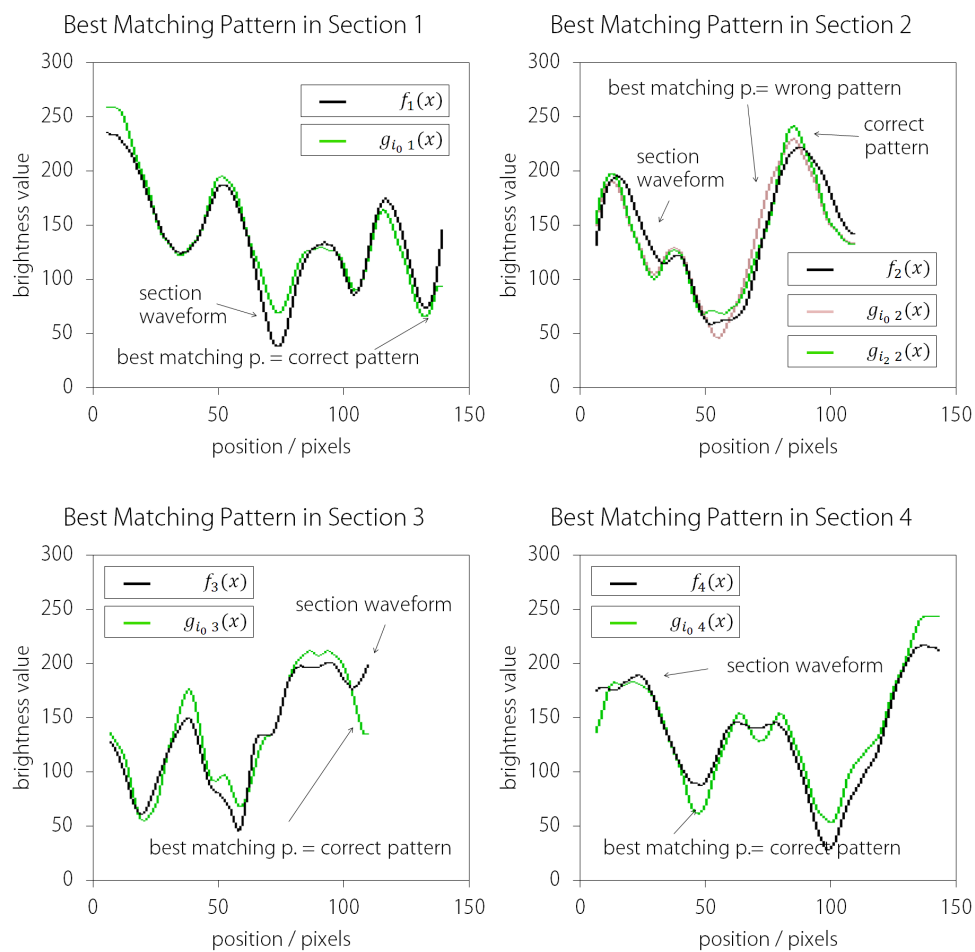
Figure 3.24 Section waveforms and their best fitting, pre-calculated patterns. In section 2, not the pattern corresponding to the correct digit and parity combination for our test code was found as the best fitting pattern, but a different one.
