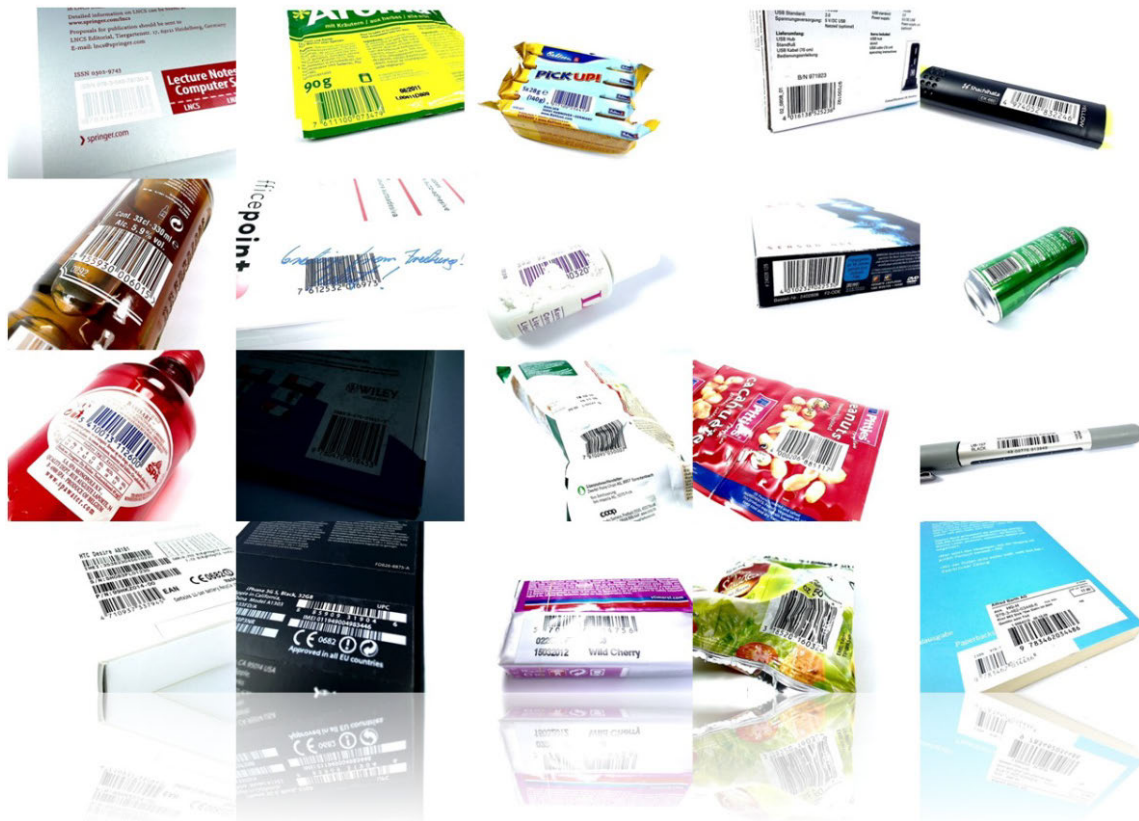
Figure 5.17 Subset showing 20 out of the 31 tested bar codes and conditions in the scanner analysis.
