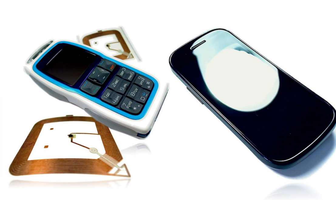
Figure 6.4 NFC/RFID tag and the Nokia 3220 device with NFC support (left image), and the Google Nexus S device with NFC support (right image).
