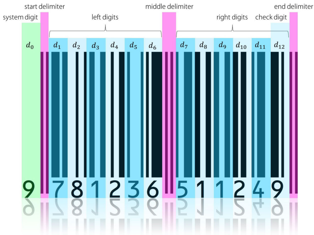
Figure 2.6 Structure of an EAN13 bar code.
