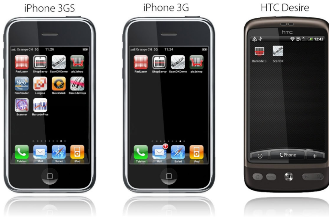
Figure 5.1 Mobile phones used for the study: An iPhone 3GS with autofocus camera (left image), iPhone 3G with a fixed-focus lens (middle image) running iOS, and the HTC Desire with a fast autofocus camera running Android OS (right image). The "ScanDK"-demo application uses our bar code recognition method.
