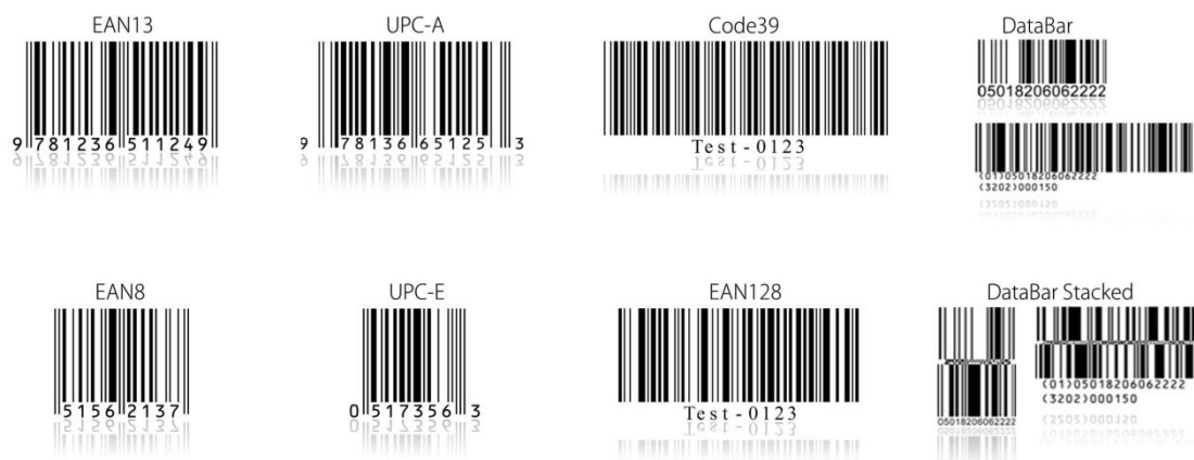
Figure 2.5 Most frequently used bar code symbologies (EAN/UPC) and future codes (DataBar).
