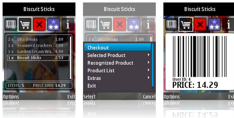
Figure 7.10 Screenshots showing the "Self-Checkout"-plugin, which allows users to manage scanned products on a list and displays a reference bar code that can be presented by users at the POS (point of sale) for self-checkout.
