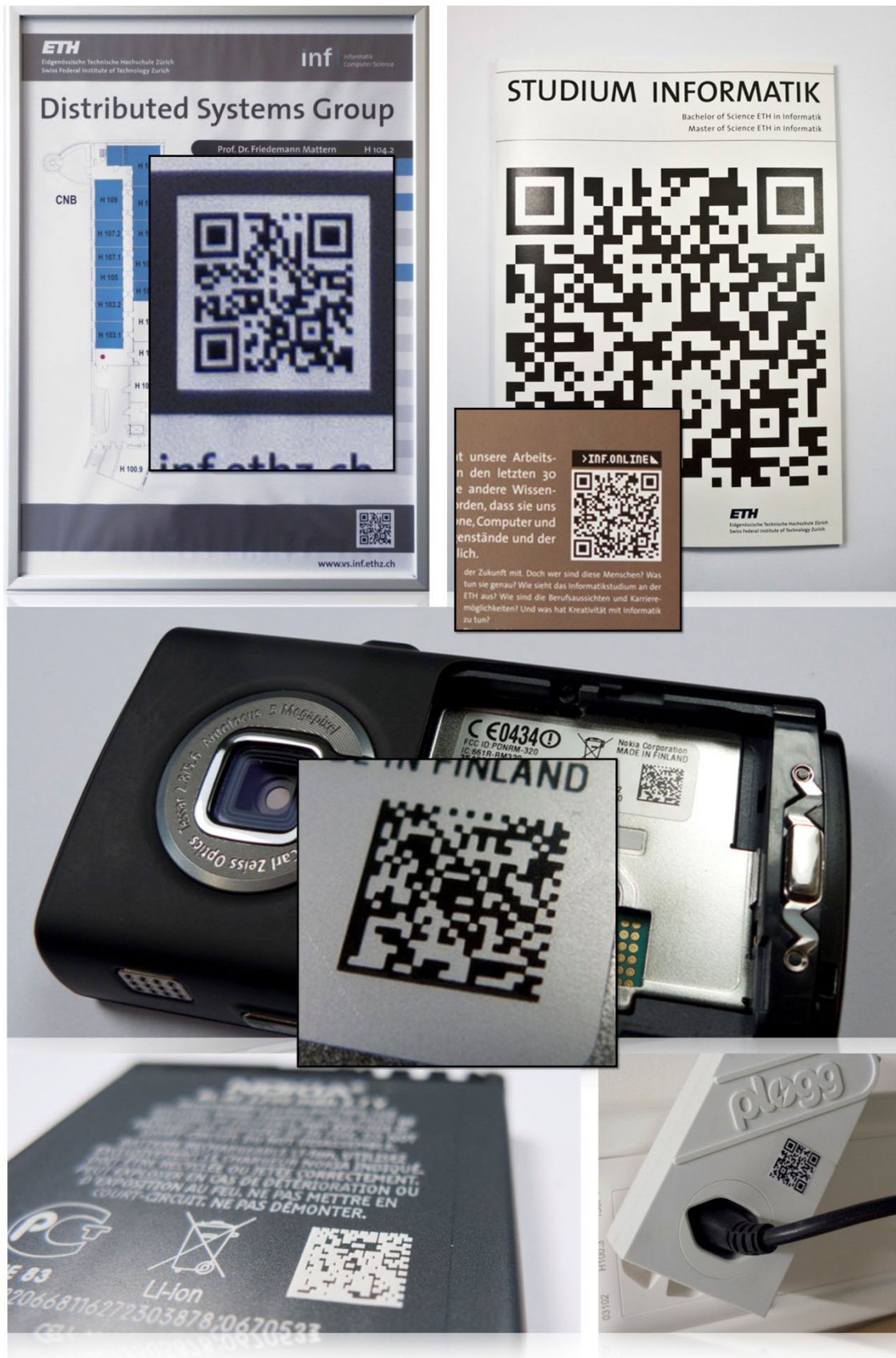
Figure 6.3 Application examples of 2D codes: posters (upper-left image), magazines (upper-right image), tagging of electronic devices (lower-left images), and for linking real-world devices to their Web-presence (lower-right image).
