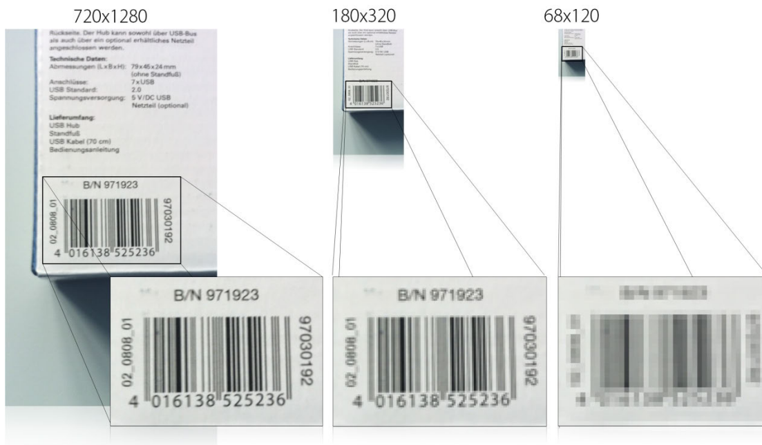
Figure 4.19 The same test image in three different resolutions and the corresponding details of the contained bar codes.
