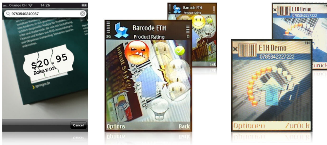
Figure 3.2 Screenshots of an augmented-reality price-check application that overlays the real camera images with a virtual price tag that changes position, orientation and size according to the bar code visible in the images (left image from an iPhone 3GS). Prototypical application illustrating orientation sensitive menus (middle images from a Nokia N95 device) and sliders (right images from a Nokia N70 device).
