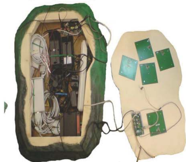
Figure 3. The Augmented Knights Castle showing internal system RFID technology, antennae (right hand side) multiplexers, and surround sound inside main section.
