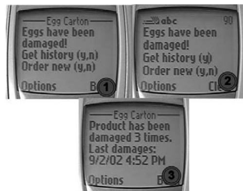
Figure 5: An SMS notification received from a smart product by a mobile phone (1), a response message with activated history command (2), and the corresponding result from the egg box (3).
