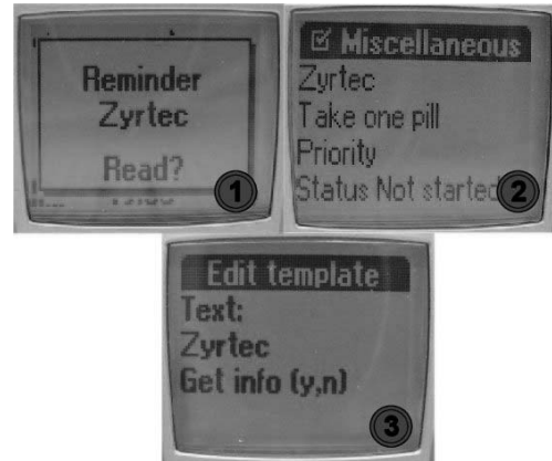
Figure 8: An alarm previously written to a mobile phone from the medicine cabinet to remind patients to take the medicine Zyrtec (1, 2), and an SMS template that can be used by a patient to get further information about this medicine by asking the virtual counterpart (3).
