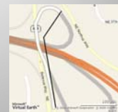
Krumm, Letchner & Horvitz, 2006 • Noisy GPS matched to road driven • Constraints from speed & road connectivity
