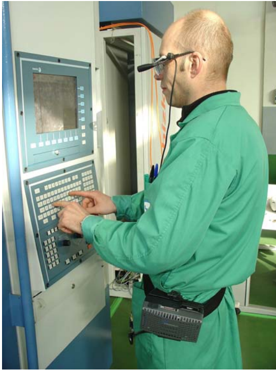
Fig.2. A worker wearing HMD connected to the Xybernaut and using the Milling Machine's CNC keyboard to interface the wearable computer
