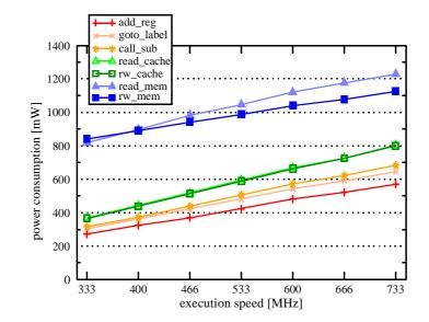
The higher the clock frequency, the higher the power consumption
