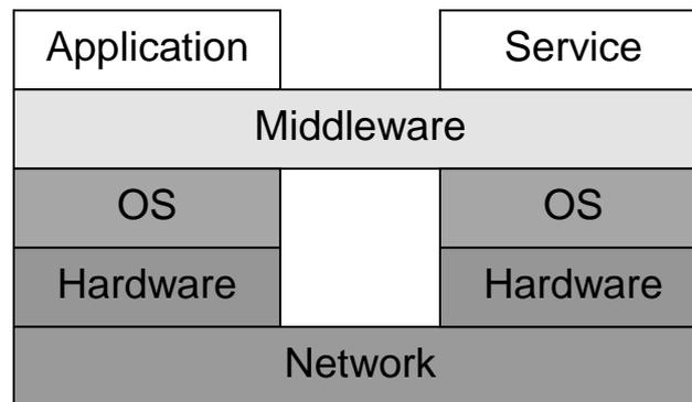
The properties and the requirements on middleware in an ubicomp environment are different from those in statically configured networks, where for example COM/DCOM and CORBA are used. Therefore there is need for new middleware suited for the new conditions.
