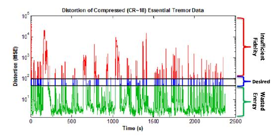
Figure 10. Dynamic distortion of movement data for a fixed compression ratio [29].
