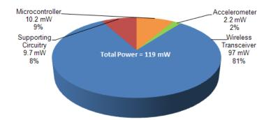
**Figure 7.** TEMPO 3.1 power consumption breakdown (with gyroscopes off).
