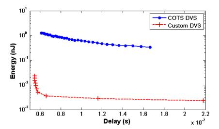
**Figure 6.** Energy-delay curves for DVS in a COTS microcontroller and a custom design.
