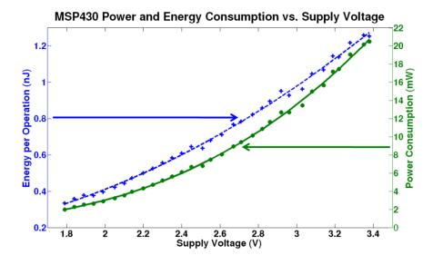
Figure 5. Operating points for a COTS MCU [9].
