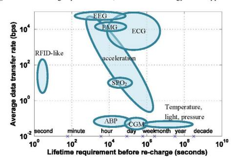
**Figure 2.** Broad design space for BSN, but size limits energy for all applications.
