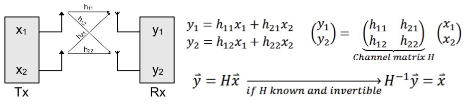
Channels are estimated by sending known preamble from each transmitter in sequence
