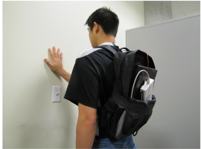
Figure 1: Participant performing a touch gesture above a light switch. The signal is measured at the participant's neck and then recorded by the data acquisition unit and a laptop in the backpack. (Image from [1])
