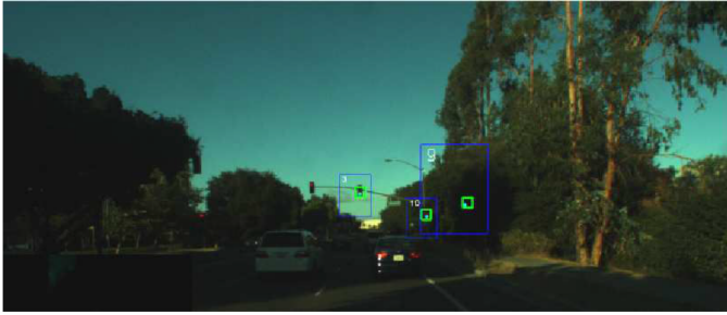
Figure 5: An example showing traffic light detection[14]
