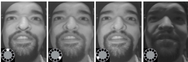
Figure 5: Four frames of input, with different LEDs active as illumination.[5]
