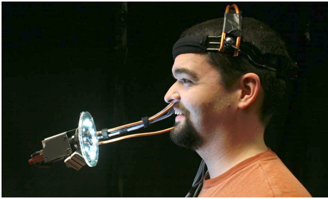
Figure 4: The camera lens is surrounded by a ring of LEDs that can be controlled individually.[5]
