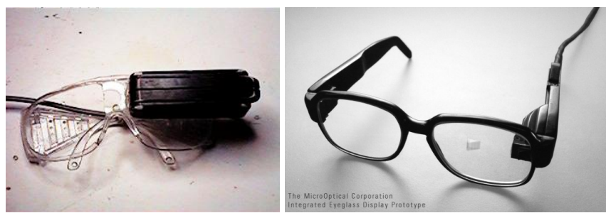
Figure 5: Wearable Display: left picture shows a PrivateEye micro-display mounted on a glass; right picture shows state of the art integrated eyeglass display.
