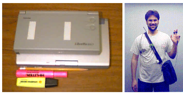
Figure 1: Left: Two Popular Mini-notebooks, Toshiba Libretto 50 (Top) and Sony PCG-C1 (Bottom). Right: A User Wearing MIT's Lizzy Design.
