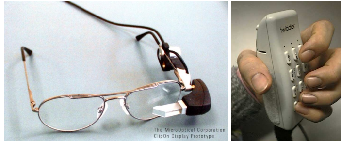
Figure 2: Typical I/O Devices: left picture is a micro-display to be clipped onto a eyeglass frame; right picture shows a twiddler keyboard with integrated mouse functionality.
