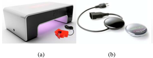
Figure 1. Display unit and sensor of Wattson (left) and Click (right).
