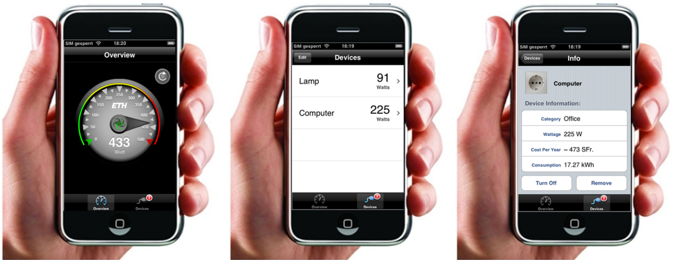
Figure 4: The mobile user interface shows the current entire consumption of all devices attached (left), a list of discovered Ploggs including their name (middle), and more detailed information per Plogg (right).
