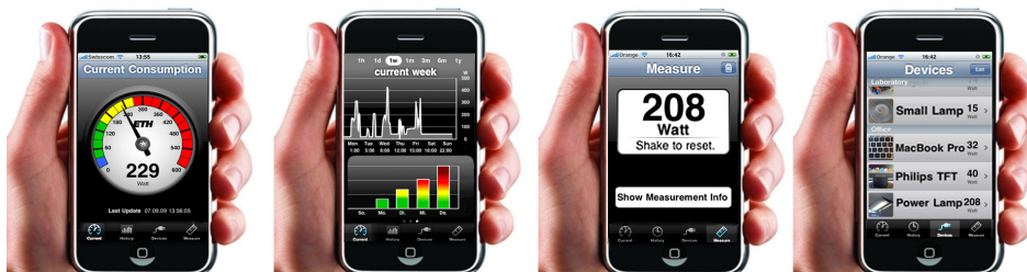
Fig. 2. The UI (left to right): Consumption view, history view, measurement view, and device inventory view.
