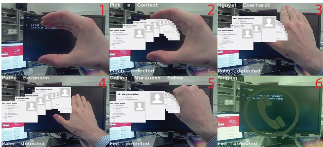
Figure 4.35: 3D gesture control in an augmented reality phone book. The user can open the phonebook by the pinch gesture (1)-(1), swipe through the contact cards by moving the hand further or closer (3)-(4), and pick a contact by grabbing it (5).
