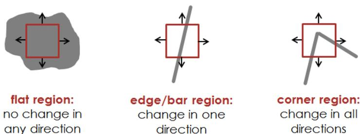
Figure 2.2: Flat, edge, and corner image areas can be distinguished by shifting a patch and comparing it with its small neighborhood. Figure adapted from [75].
