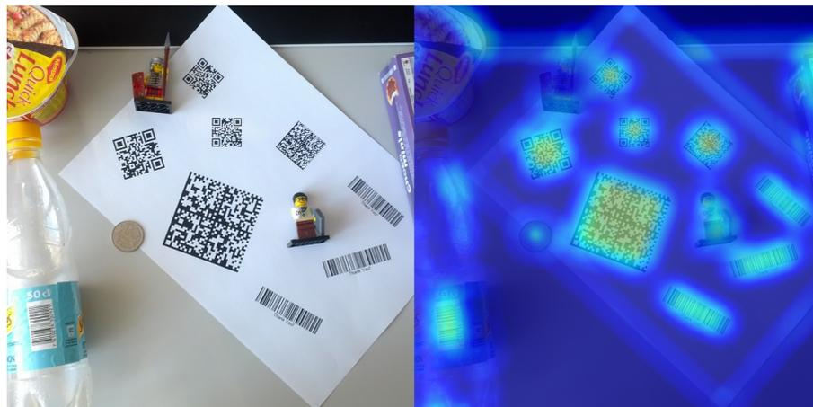
Figure 1.14: Our localization method is able to detect 1D and 2D symbologies at various scales. Left: input image. Right: code probability map overlaid on the image
