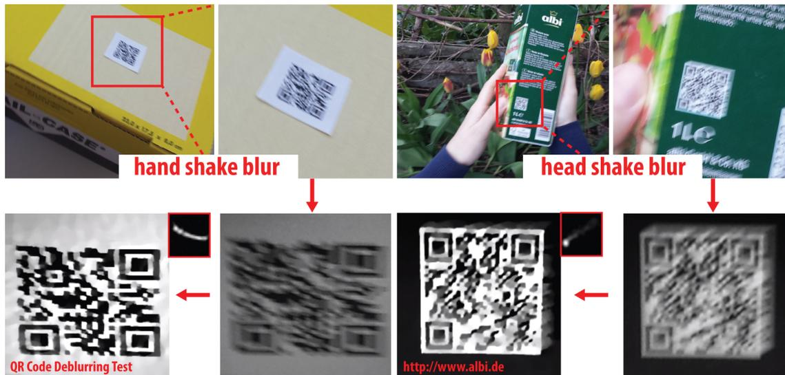
Figure 1.15: Top: When the camera or the scanned object move even slightly during scanning, the captured visual codes become distorted by motion blur and conventional decoder algorithms cannot decode them. Bottom: We propose a fast blur removal algorithm that allows the scanning of motion-blurred QR codes.
