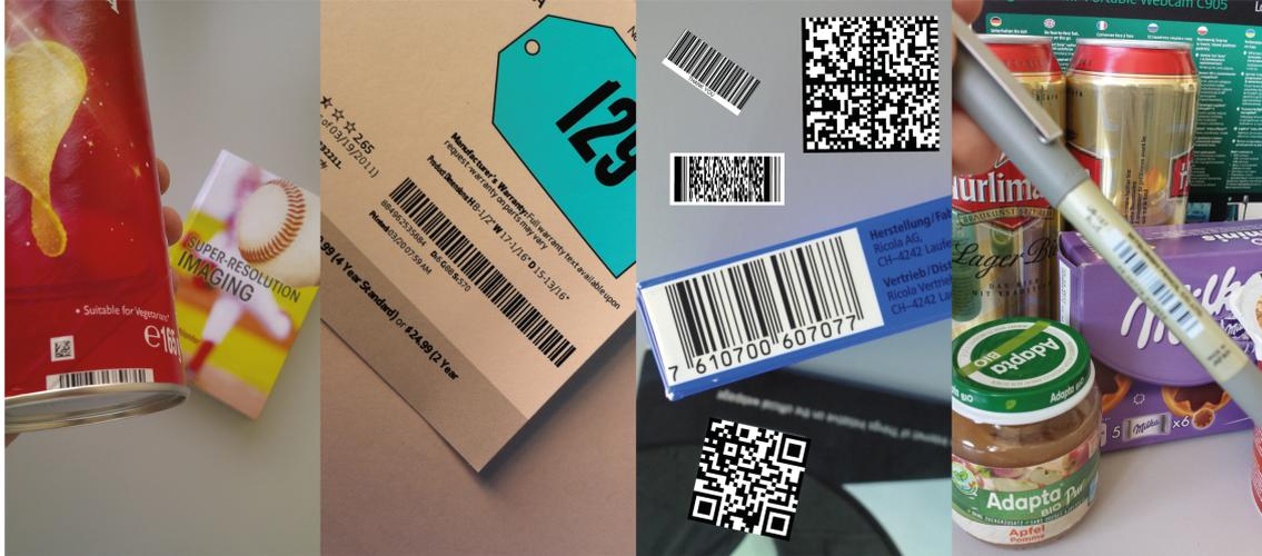
Figure 2.1: Visual code localization in digital images poses *four main challenges*: different scales, different orientations, different symbologies, blur.
