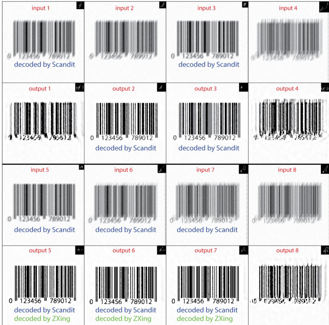
Figure 3.23: Experiment with a  $300 \times 300$  barcode image and synthetic blurs with the kernels of Levin [133]. Here the blur is visually smaller than in Figure 3.22. Again, our method makes some barcodes decodable with ZXing, but some codes become even worse than the input, and the Scandit scanner can actually decode the ones where the motion blur can be approximated by a defocus blur model.
