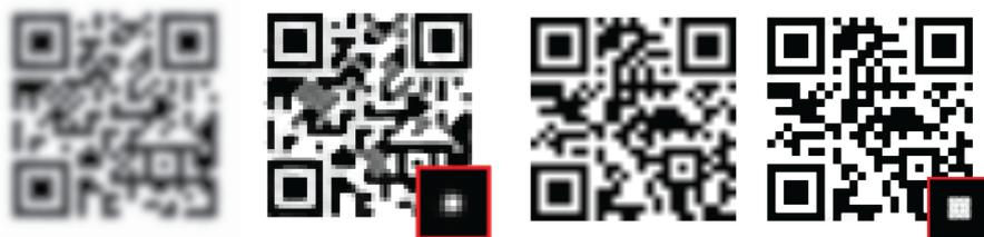
Figure 3.24: Left: removing synthetic defocus blur. Note the Gaussian-shaped estimated kernel. Right: Reconstructing a bilinearly  $12\times$  upscaled code. Note the square-shaped estimated kernel.
