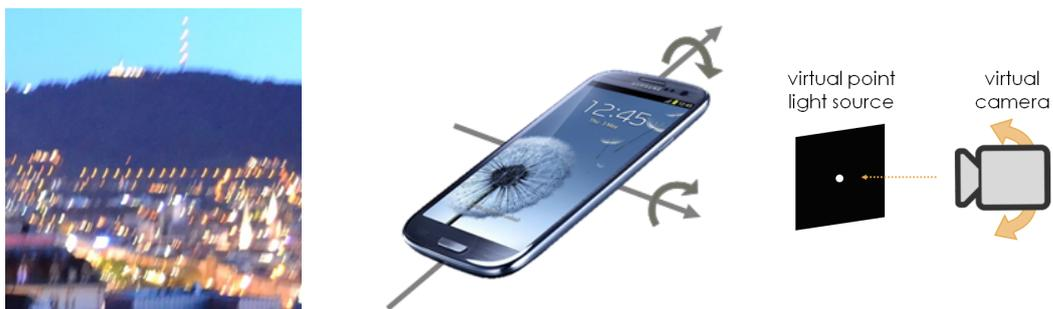
Figure 3.27: Left: The blur is “encoded” in the image of point light sources. Middle: We can reconstruct the camera motion from inertial sensor measurements. Right: We can get the blur kernel by replaying the motion with a virtual camera looking at a virtual point light source.
