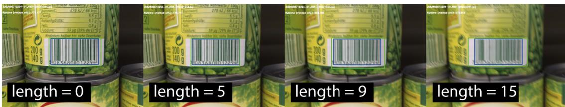
Figure 2.10: Successful 1D detection rates ( $J \geq 0.5$ ) on 1000 images from the Muenster data set with various degrees of artificial motion blur. The bottom row gives an impression on the effect of the blur length.
