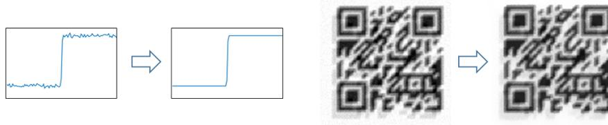
Figure 3.9: The weighted median filter smooths high-frequency components but keeps sharp edges.
