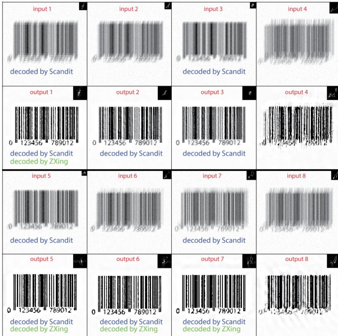
Figure 3.22: Experiment with a  $200 \times 200$  barcode image and synthetic blurs with the kernels of Levin [133]. Our method can make 4 out of 8 images decodable with the simple ZXing decoder. However, some codes degraded by small (or concentrated) motion blur can be decoded with the Scandit scanner that applies a very efficient defocus blur model.
