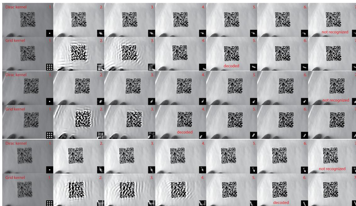
Figure 3.20: Further examples illustrating image and kernel refinement using a single peak or a grid of peaks as starting kernel. In these examples, codes were not recognized using the peak initial kernel, but our grid kernel is successful in removing large blurs.
