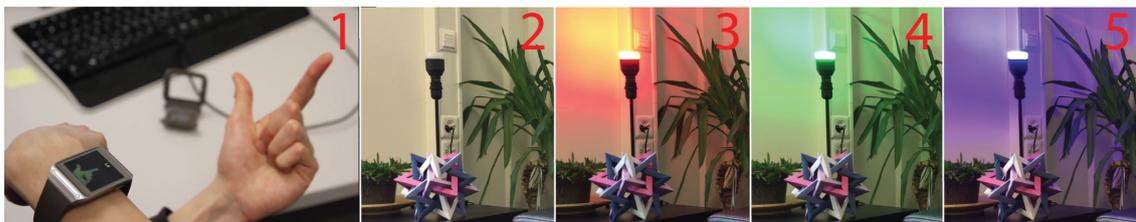
Figure 4.33: Controlling a Web-enabled light bulb with simple gestures performed around the smartwatch. The subsequent gun and pointing gestures change the color of the light.
