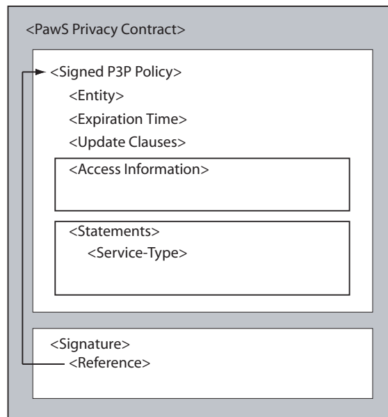
Figure 4.5: PawS privacy contract . Privacy contracts consist of a regular, optionally signed P3P policy with a number of PawS specific extensions, such as access methods, service type information, and additional data schemas particular to ubiquitous computing environments.
