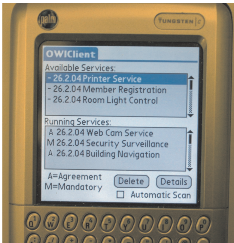
Figure 4.21: Privacy assistant main interface , as implemented on a Palm PDA. It shows the services for which a privacy contract has been received from a beacon, as well as a list of currently active services.
