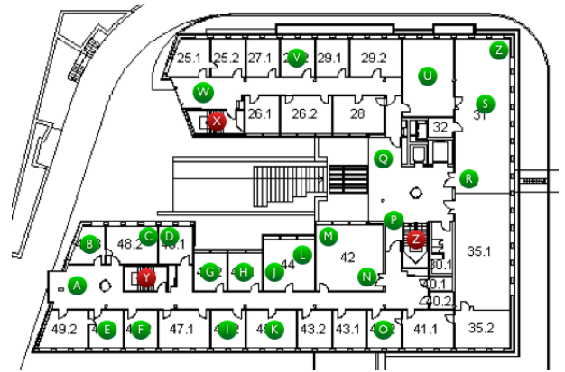
Figure 5: Points where measurements were taken. The labels A to W indicate on-floor measurements while X, Y, and Z indicate measurements that were taken on the stairs between the floors.
