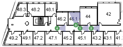
Figure 6: Cameras setup in triangle.
