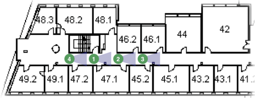
Figure 5: Linear camera setup in a hallway.
