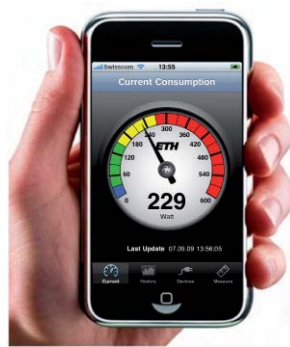
Figure 1: Live visualization of current household electricity consumption
