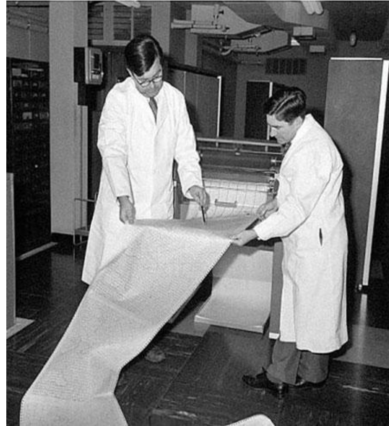
Weather-forecast printer, Meteorological Office, 2 November 1965: Charles Jarvis and Ray Belton, operators of the high speed line printer, hold a length of forecast charts which the computer-fed machine produces at 1000 lines a minute.
