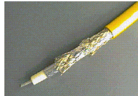
Ethernet yellow cable
