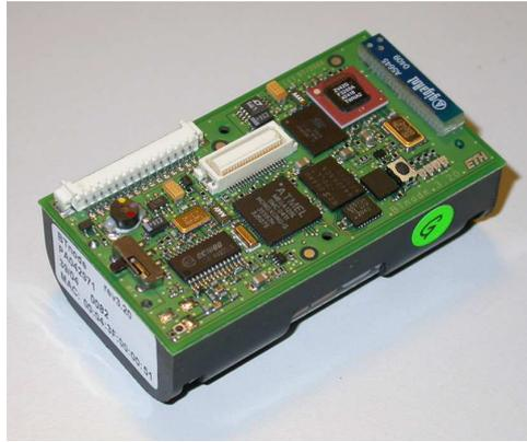
**Figure 2:** Example of a sensor node: BTNode.
