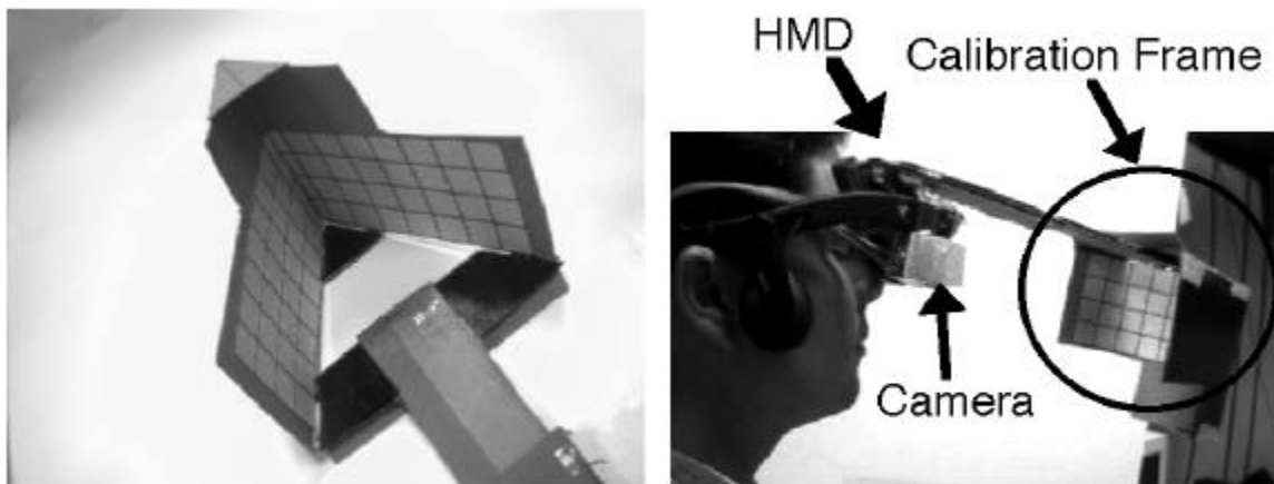
Figure 18. The Calibration Frame used in our Calibration Method.
