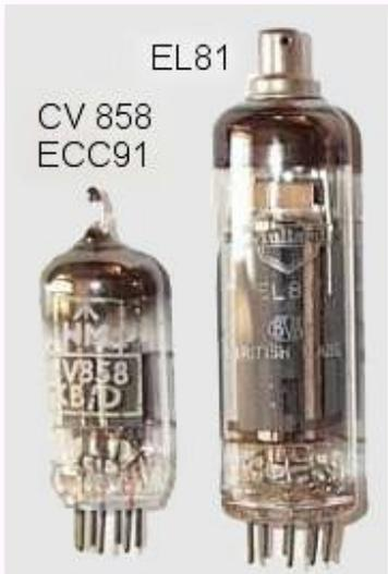
“...valves of nine types, of which the most common was the ECC91 common-cathode double-triode. Another was the EL81, which was used to drive the head movement on the drums. The failure rate of valves was typically about 40,000 hours, so with 1400-odd valves in Deuce it doesn't take a genius to work out that they failed fairly frequently.” [P.J. Walker]
