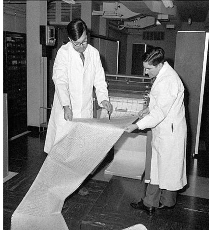
Weather-forecast printer, Meteorological Office, 2 November 1965: Operators of the high speed line printer holding a length of forecast charts which the computer-fed machine produces at 1000 lines a minute.
