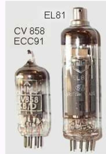
"...valves of nine types, of which the most common was the ECC91 common-cathode double-triode. Another was the EL81, which was used to drive the head movement on the drums. The failure rate of valves was typically about 40,000 hours, so with 1400-odd valves in Deuce it doesn't take a genius to work out that they failed fairly frequently." [P.J. Walker]
