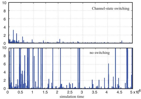
**Figure 4: Simulation history of a wireless networked control system whose dropouts following a two-state Markov chain. The top plot shows the response of a channel-aware switching controller and the bottom plot shows the response of a controller that does not switch on channel state.**
