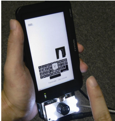
In-air typing interface for mobile devices with vibration feedback [Niikura et al. SIGGRAPH 2010]
