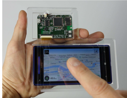
A low-cost transparent electric field sensor for 3D interaction [Le Goc et al. CHI 2014]
