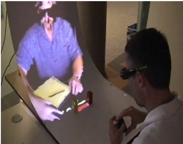
Figure 7: MirageTable [2]. A projector and a Kinect are located on top of the curved surface, looking down on the user. Image from http://www.engadget.com/2012/05/12/microsoft-researchs-miragetable-brings-some-augmented-reality-t/ .
