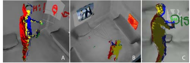
Figure 13: A) and B) Flashlight-like metaphor: Virtual drawings or images are associated with a certain location. C) The user "draws" in 3D, while virtual shadows are projected.
