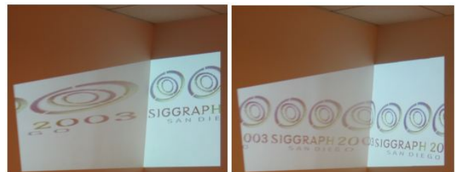
Figure 4: Distortion correction for an image projected onto a non-planar surface.
