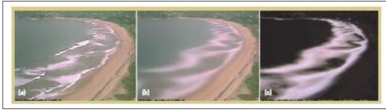
Fig. 1. Palm Beach, Australia: (a) snapshot, (b) 10-minute time exposure, and (c) variance image. [1]
