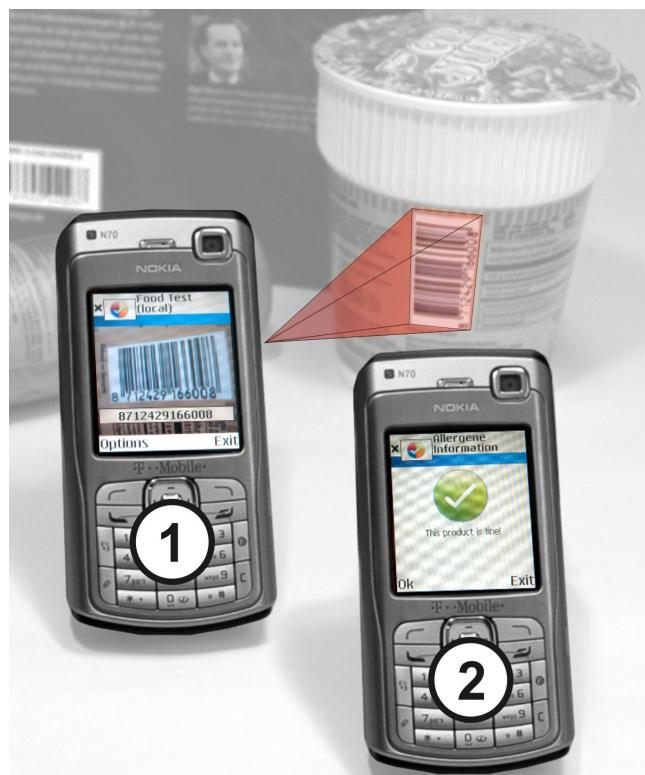
Fig. 3. Robust scanning of bar codes with camera-equipped mobile phones.
