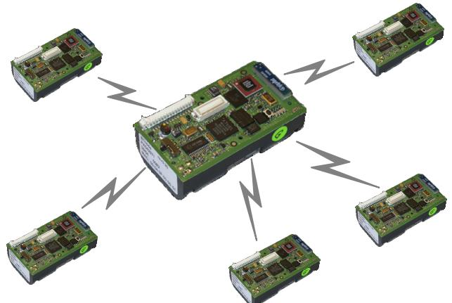
Fig. 2. BTnode: a hardware and software platform for sensor networks.
